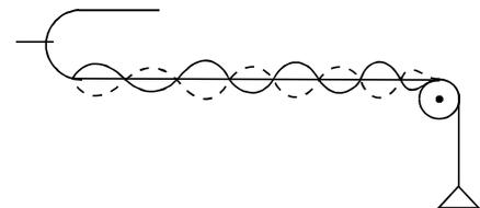
(1) **Transverse arrangement** : Oscillations of tuning fork are set perpendicular to length of string frequency of tuning fork and of waves on string are same so if  $n$  is number of loops in string then
